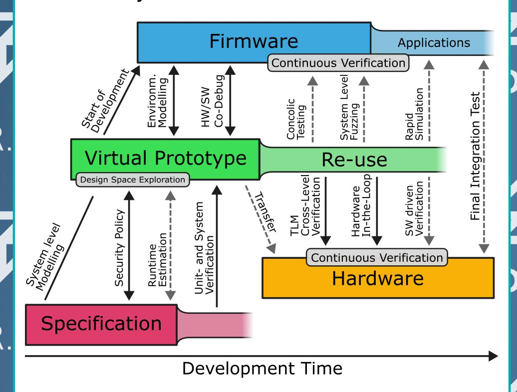
The speedup mainly relies on the HW/SW codevelopment (shift left principle) and early design space exploration. This allows problems like HW-SW-Partitioning [6] to be solved **before** the existing design can't be changed.
