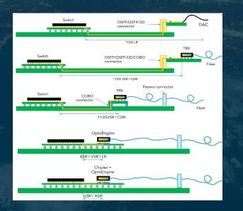
Digital Interfacing Technology – Optical Transceivers
