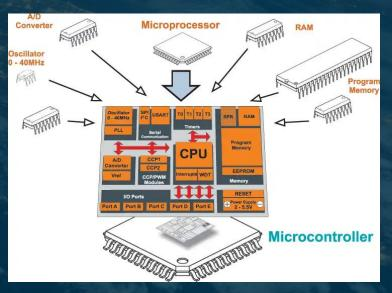
Embedded Computing Technology - Microcontroller
