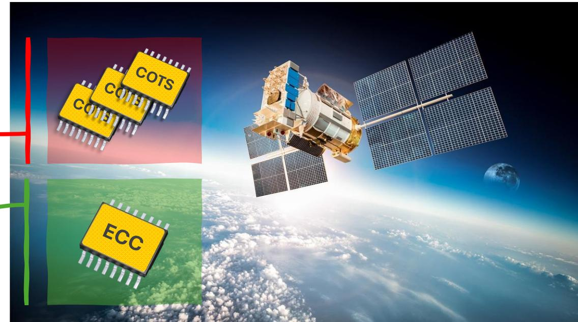
**Electronics systems for Space** applications are exposed to **extreme conditions**, leading to a variety of **HW errors**, such as: **SEU (Single-Event Upset)**, **SET (Single-Event Transient)**, **SEL (Single-Event Latch-up)**
