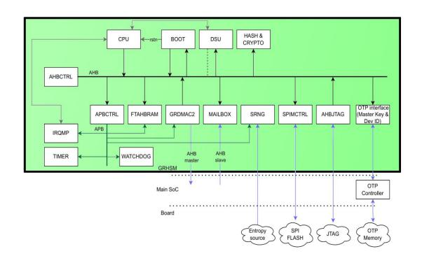
• Separate SoC with private external SPI flash storage that interfaces the rest of the system via a mailbox interface. Independent execution after device reset.
