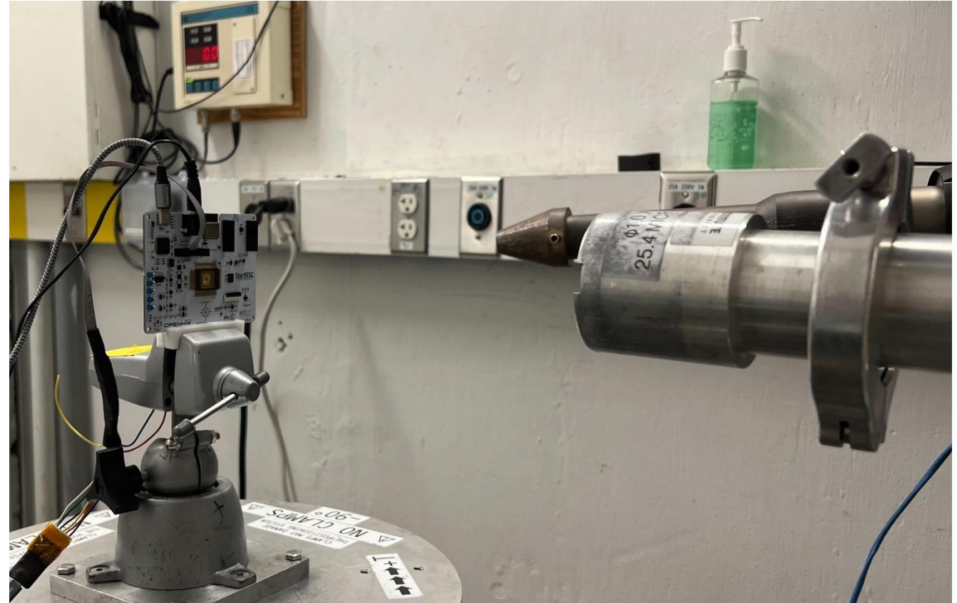
StarRISC undergoing Heavy Ion Testing @ TAMU
