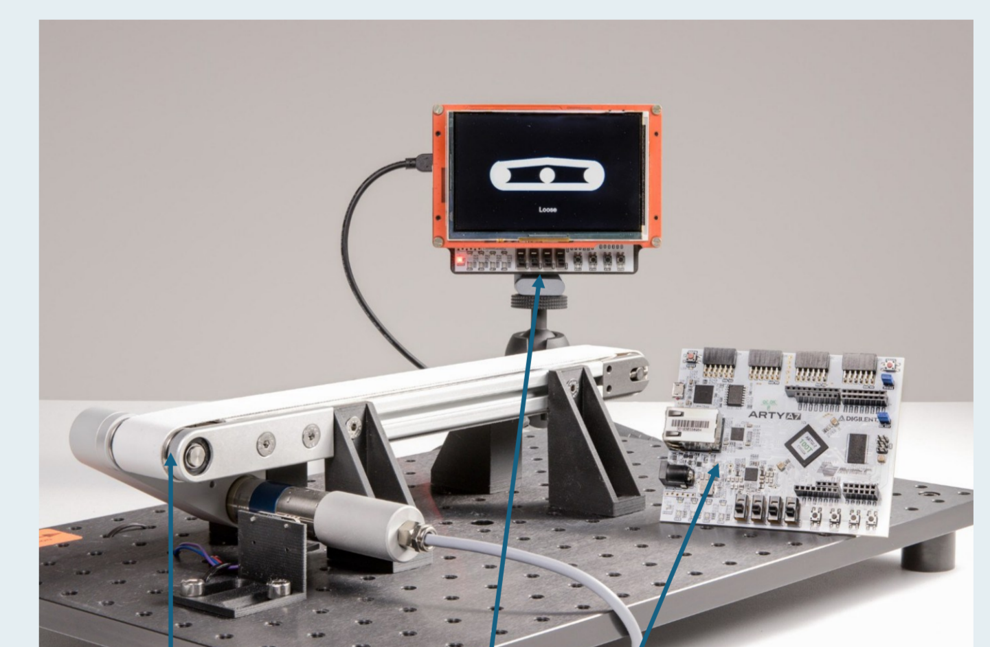
Integrated Sensors, FPGA based platform (with Display), EMSA5 EMMI (AI Framework)
